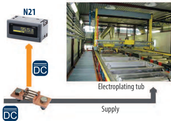
Current measurement in an electroplating plant
