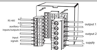
Fig.86 Connection of input signals
