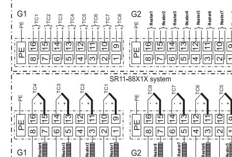
Fig. 101 Way of SR11 system external connections
