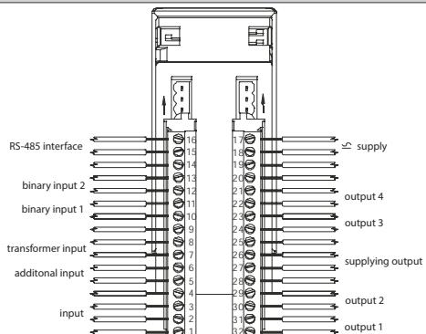
Fig.90 Connection of input signals
