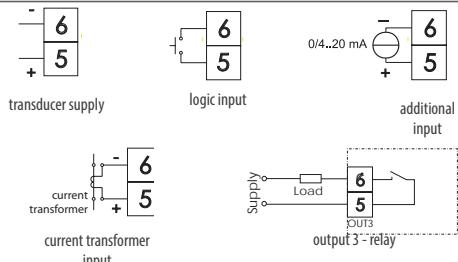
Fig.88 Connection of load circuit
